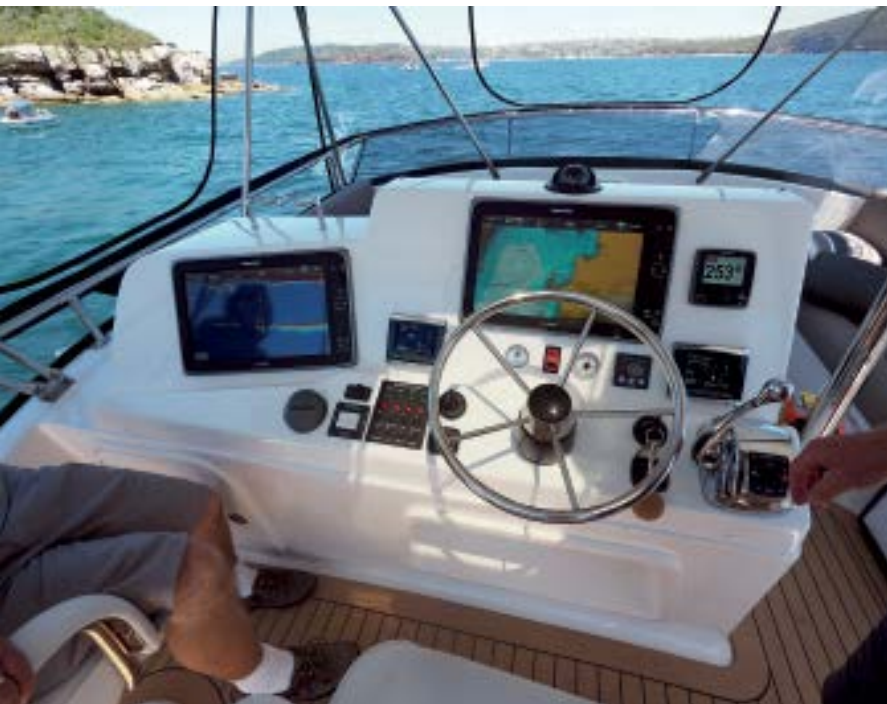
Above: The wide dash features a pair of 40cm Raymarine screens connected to a Raymarine 470 1kw dual range CHIRP sounder module, a Navionics Platinum map card and a 48NM radar.
